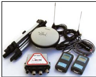
GPS-Base components, here shown with SATEL radio modems.
