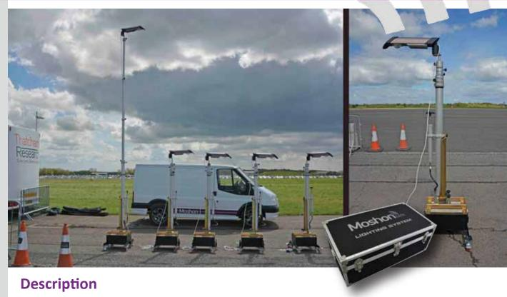
The new MD-SL NCAP lighting system is a complete 5-streetlamp system designed and tailored specifically for the NCAP AEB VRU night testing procedure.
