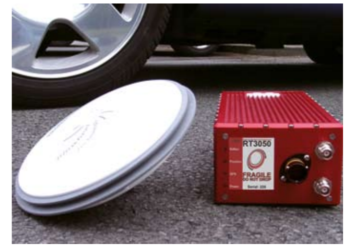
Team GRAY gets underway (above). The OxTS-developed RT3000 series (RT3050 shown below) inertial and GPS navigation system, successfully used in the DARPA Urban Challenge
