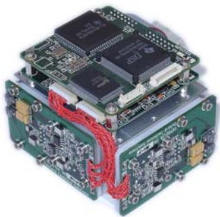
Inertial Sensors in RT4000 include servo-grade accelerometers and precision MEMS angular rate sensors. Powerful 40MHz floating point DSP takes care of coning, sculling and aliasing.
