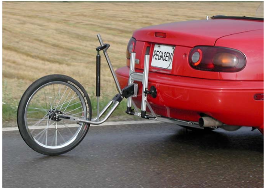
5 th -wheel 5W-20 in action attached with elements from the FMS Mounting System.
