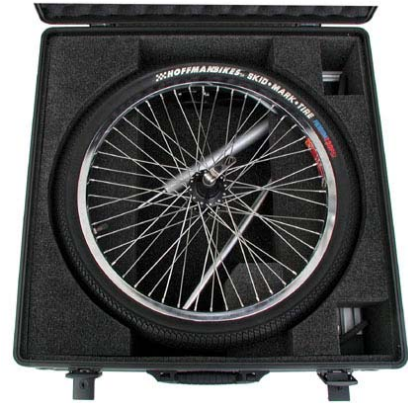
The 5th wheel with accessories perfectly fits into the custom-made transportation case. 550x550x250 (WxDxH)
